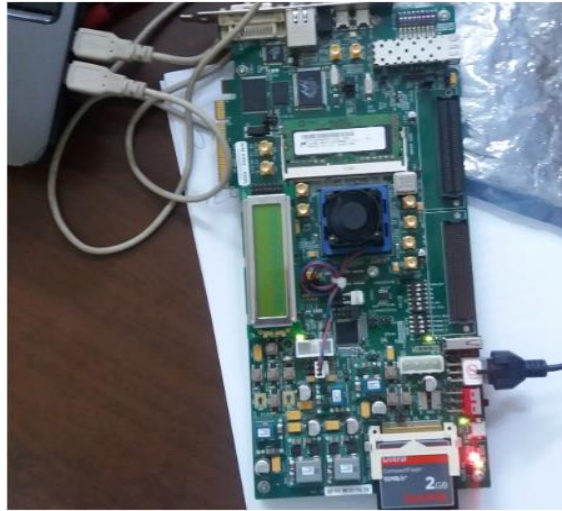
Fig. 8. FPGA Kit for Virtex 6 (XC6VLX240T).
