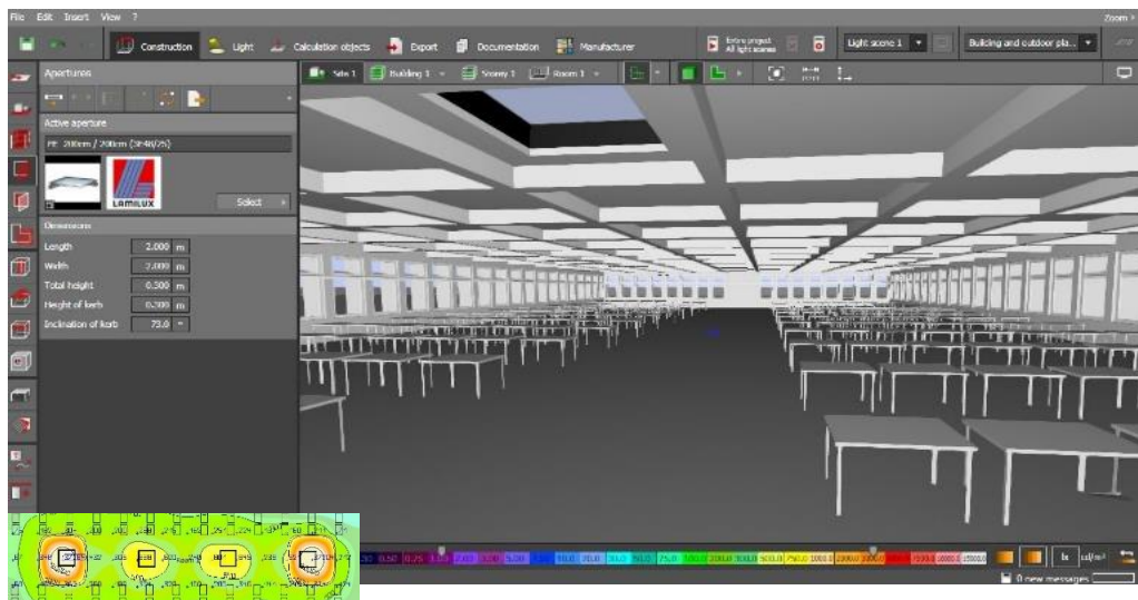
Fig. 11 Lighting distribution in the space after adding a light shelf and skylight using Dialux simulation program source: authors
